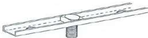
Fig. 5.6. Bolt retainer channel.
